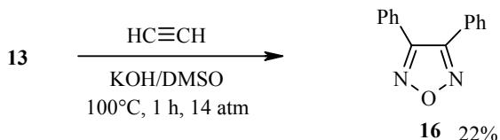
Under the same conditions in the absence of acetylene  $\alpha$ -benzil dioxime **13** is inert and does not form the oxadiazole **16**. Radicals generated during the dissociation of the obtained O-vinyloxime derivatives are probably involved in the cyclization.
