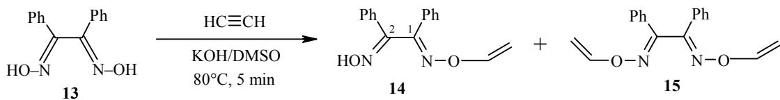
The highest yields of compounds **14** and **15** (50 and 12% respectively) were obtained at a reaction temperature of 80°C (initial acetylene pressure 14 atm) and reaction time ~5 min. If the reaction time is increased to 1 h (80°C) under these conditions or the temperature is raised to 100°C (~5 min) 3,4-diphenyl-1,2,5-oxadiazole (**16**) is formed, while the vinyl derivatives **14** and **5** cannot be isolated.
